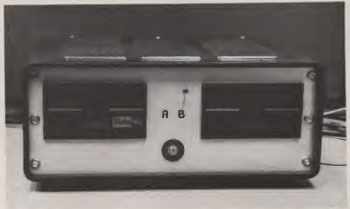
Vista dual disk drives mounted in enclosure.
